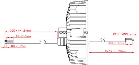
Input Cable: protect wire of black rubber, OD: Φ7.2mm, 3 x 1mm2, protruded lengths: 350mm Output Cable: protect wire of black rubber, OD: Φ7.2mm, 2 x 1mm2, protruded lengths: 240mm
