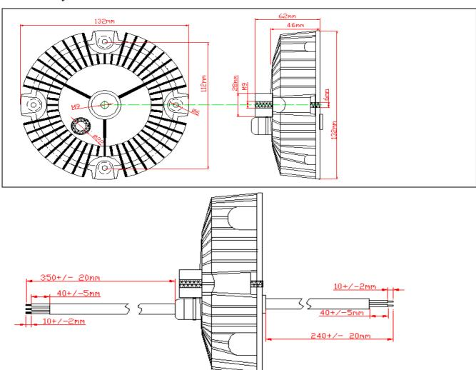
Input Cable: protect wire of black rubber, OD: Φ7.2mm, 3 x 1mm2, protruded lengths: 350mm Output Cable: protect wire of black rubber, OD: Φ7.2mm, 2 x 1mm2, protruded lengths: 240mm
